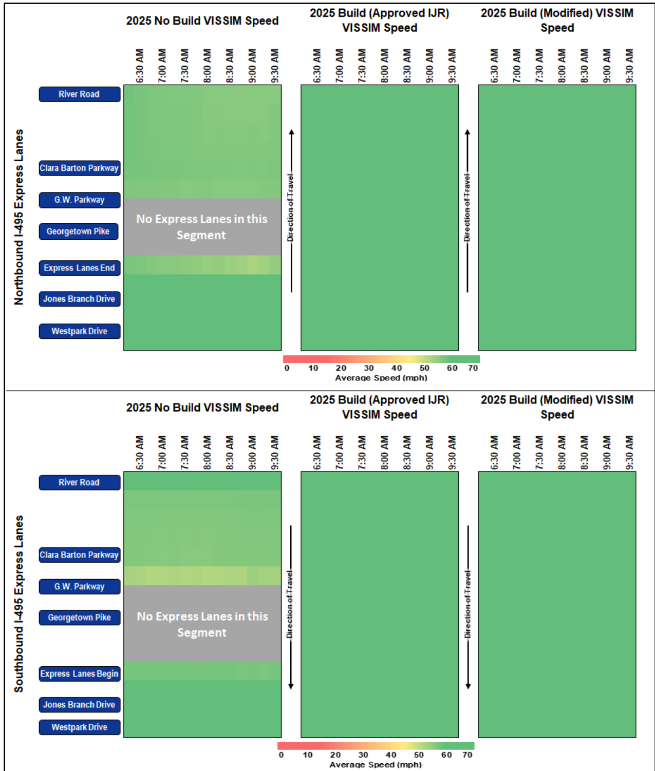
Figure 6-2. AM Peak Period Average Speeds along I-495 Express Lanes for 2025 No Build, 2025 Build (Approved IJR), and 2025 Build (Modified) Conditions
