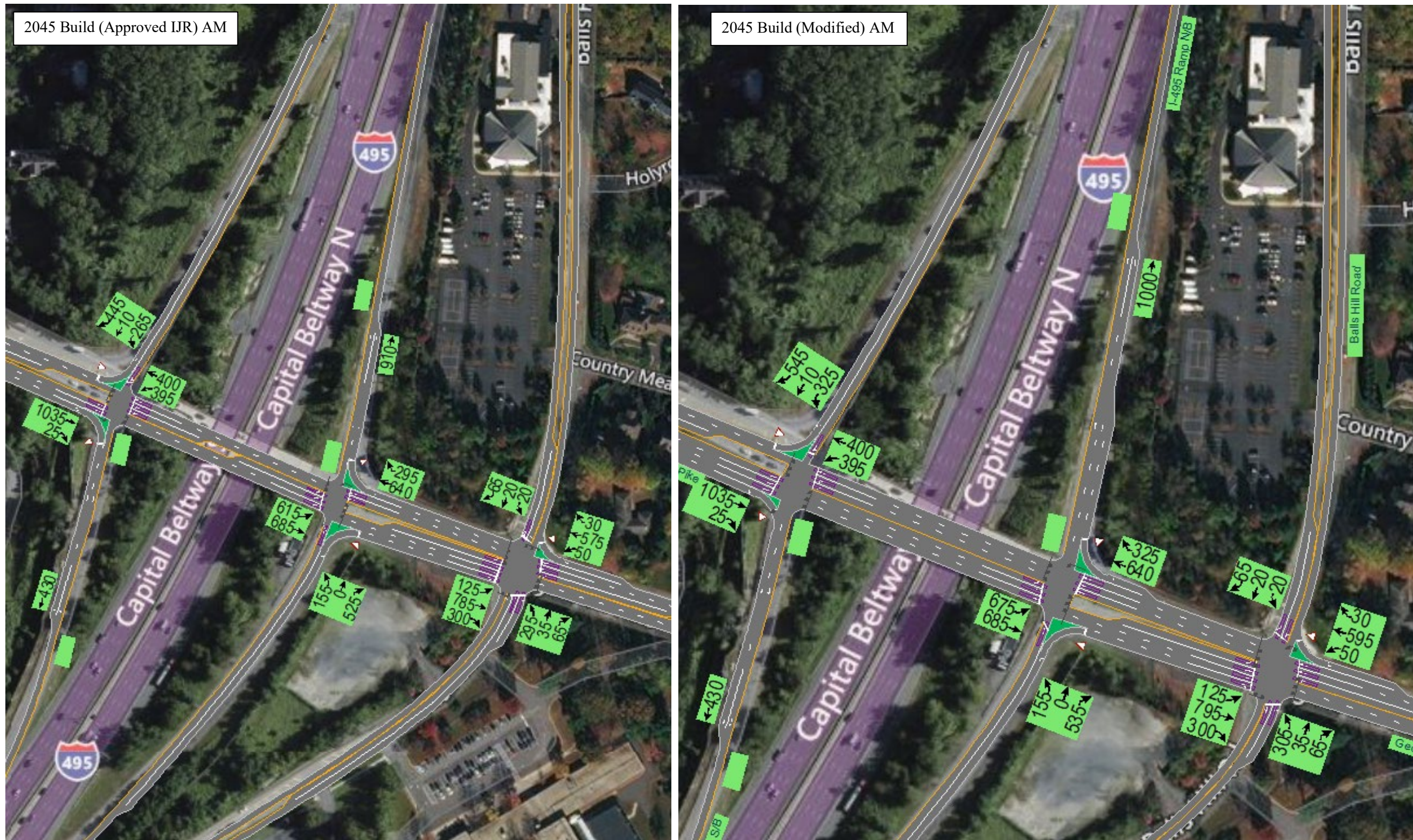
Exhibit 5-2d. 2045 Build (Approved IJR) vs. 2045 Build (Modified) Arterial Turning Movement Forecasts for IJR Addendum Study Area – AM Peak Hour
