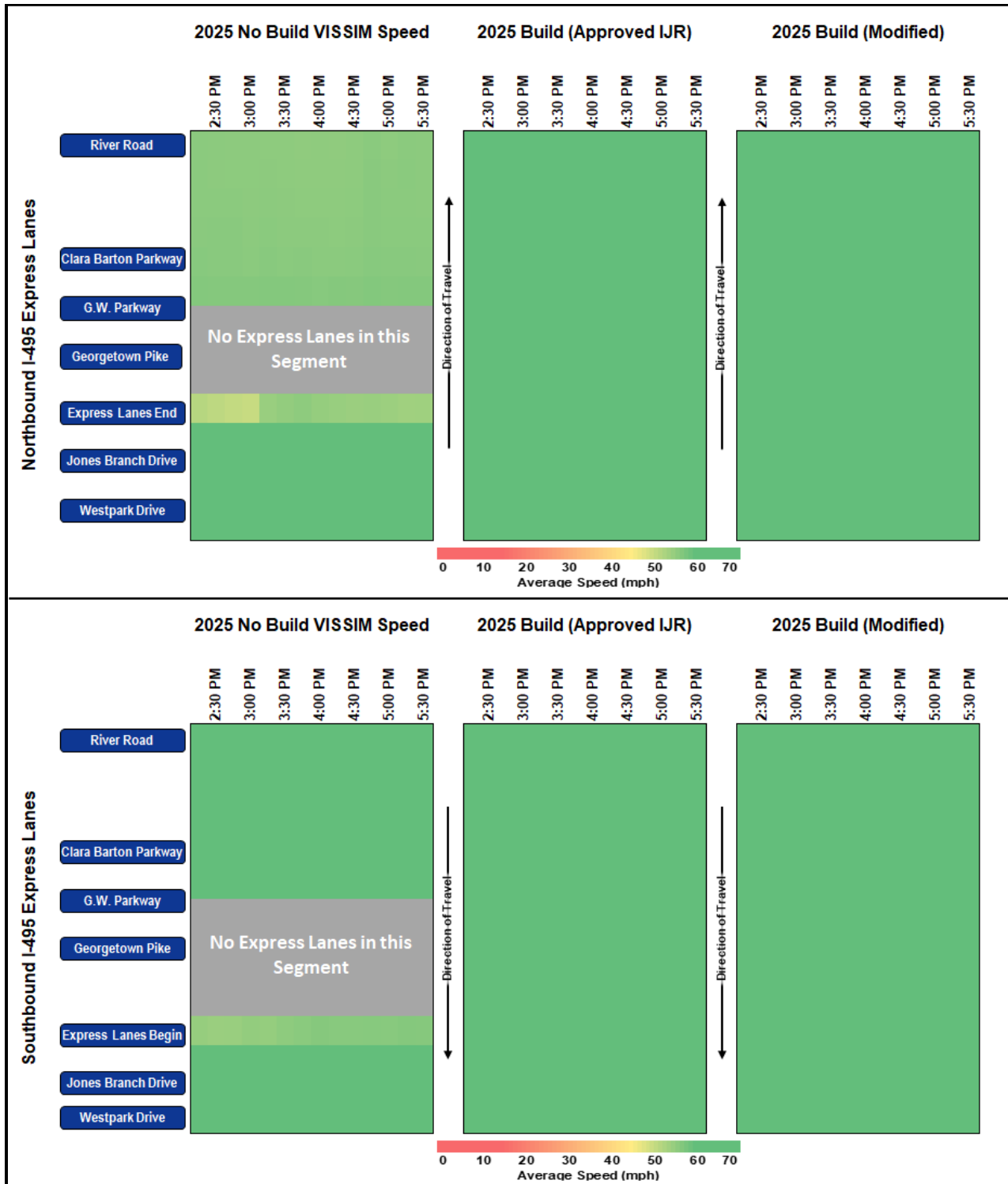
Figure 6-6. PM Peak Period Average Speeds along I-495 Express Lanes for 2025 No Build, 2025 Build (Approved IJR), and 2025 Build (Modified) Conditions
