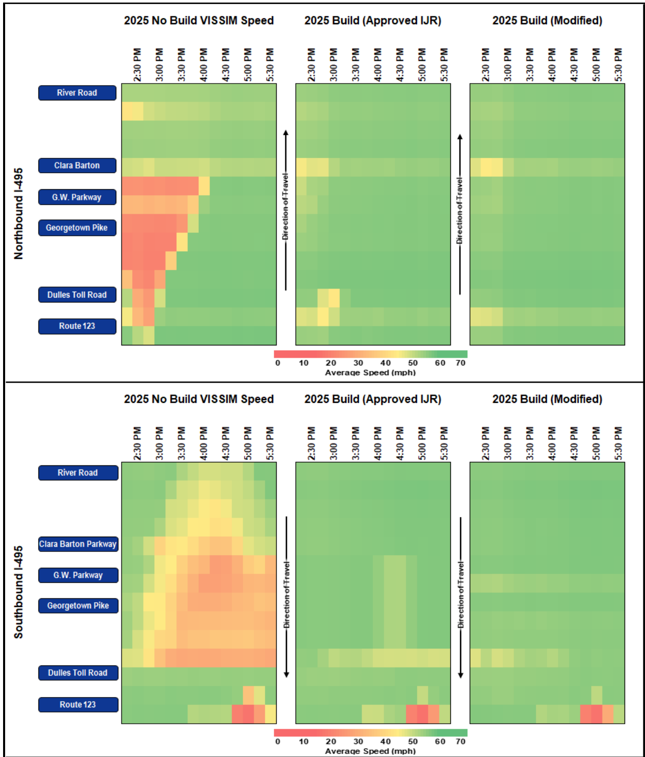
Figure 6-5. PM Peak Period Average Speeds along I-495 GP Lanes for 2025 No Build, 2025 Build (Approved IJR), and 2025 Build (Modified) Conditions
