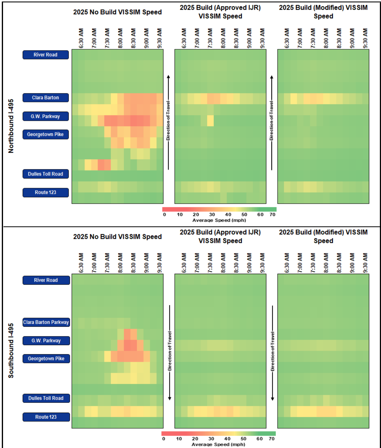
Figure 6-1. AM Peak Period Average Speeds along I-495 GP Lanes for 2025 No Build, 2025 Build (Approved IJR), and 2025 Build (Modified) Conditions
