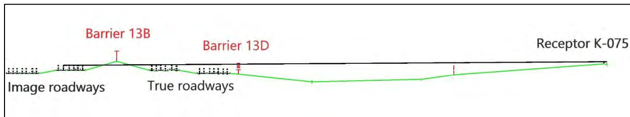
Figure 3 Cross-section at Receptor K-075 showing sound path from image roadway “misses” the reflecting surface
